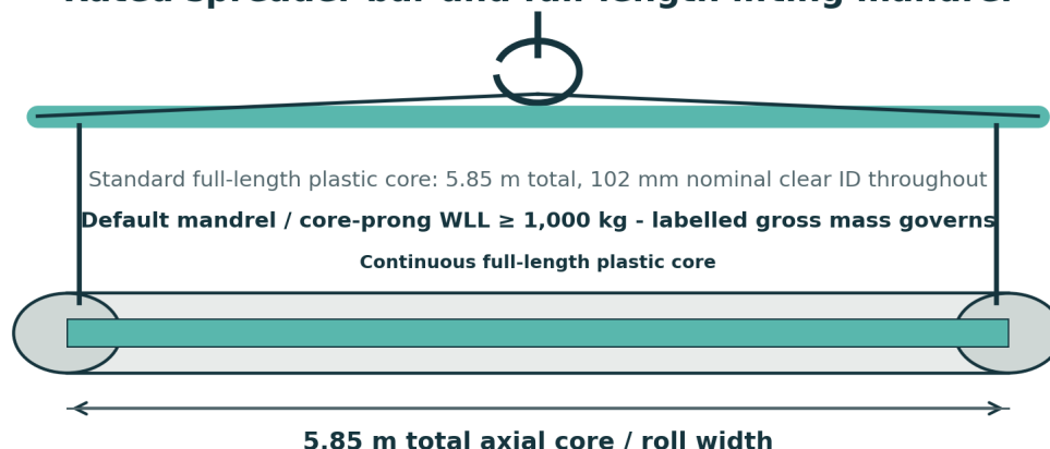
Figure 2. Minimum handling concept for a 5.85 m-wide roll.
